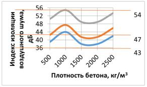
*Figure 1. Relationship between concrete density and airborne noise insulation index*
