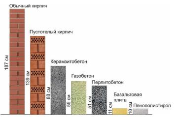
**Figure 1.** Thicknesses of various materials that provide thermal characteristics of external walls for the conditions of Almaty according to the standards adopted in 2001 (addition to SNiP II-3-79\* "Construction Heat Engineering")
