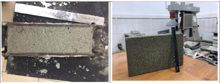
Figure 2. Perlite cement samples
